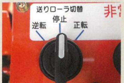
It is possible to easily reverse the Feed Roller with this switch when the machine cannot handle the feed during grinding.
