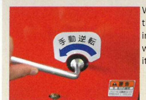
When the machine stops with the blade/hammer jammed, insert the wrench which comes with the machines and rotate it for easy release.
