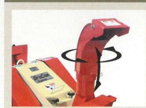
The tip can be adjusted at any angle freely so the discharge direction can be changed with ease.
