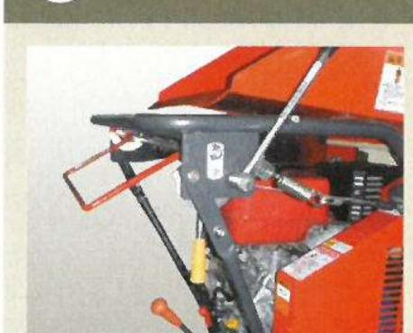
When a certain amount of force is applied when reversing, the clutch turns off and stops to prevent accidents involving crushing objects which are in the path of the machine.
