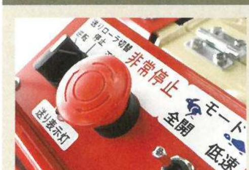
Push the emergency stop button in a emergency to stop the feed roller and engine for preventing accidents.
