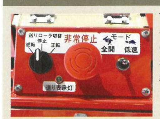
The rotor load is instantly detected automatically controlling the feed roller so you can carry out grinding with ease.
