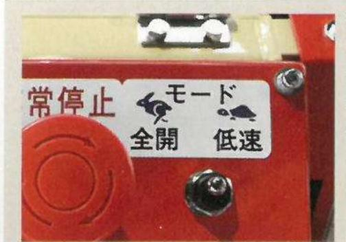
When feeding a small amount of materials such as thin branches with a diameter of 3cm or less or grass, switch to the "Thin Branch" mode to improve fuel efficiency and reduce the noise level.
