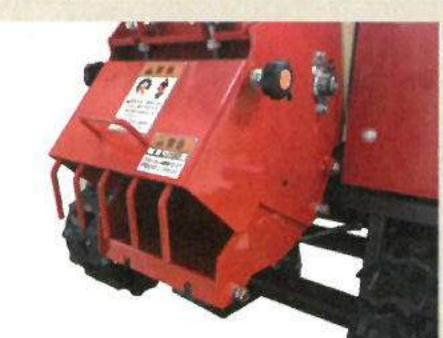
For models with a blower, use it when it is not necessary to project the tip to a distant place, or when the blower does not fly well and becomes clogged depending on the material and condition of the crushed material.
